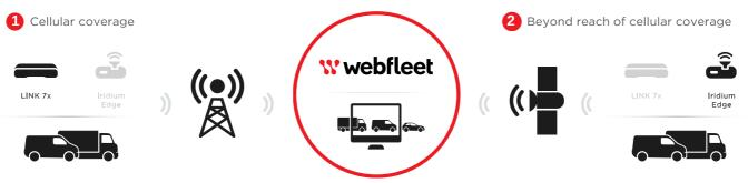
In cellular coverage areas, the LINK device transmits data live directly to WEBFLEET2.
